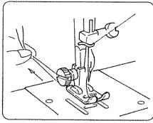
Pull both threads under and to the back of the presser foot, leaving 3 to 4 inches of thread clear.
